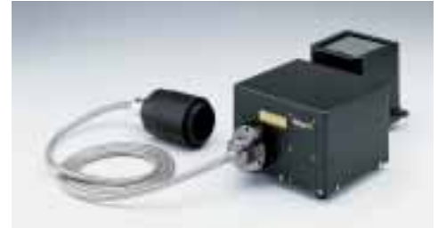
Transmitted light detection module External transmitted light photomultiplier detector and 100W Halogen conventional illumination, integrated for both laser scanning and conventional transmitted light Nomarski DIC observation. Motorized exchange between transmitted light illumination and laser detection. Simultaneous multi-channel confocal fluorescence image and transmitted DIC acquisition enabled.
