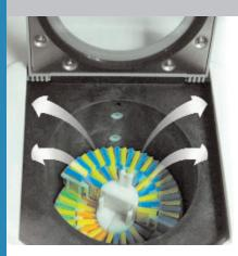
In the state-of-the-art reaction chamber, reagent circulates freely around specimens, with downdraft fume extraction.
