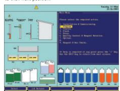
**2nd processing run:** the fresh reagents are drawn into the reaction chamber when needed during processing and placed into their appropriate bottles when the step is complete.
