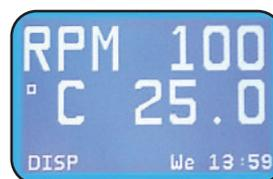
**Large, easy-to-read display screen** clearly shows operating parameters and actual value. Displayed parameters can be selected by user. A single knob selects all operating conditions easily and quickly. Screen size: 5" x 2<sup>3</sup>/<sub>4</sub>" (12.7 x 6.98 cm).
