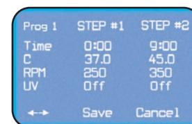
**Programmable controller** automates parameter changes on a timed basis. Holds up to 4 programs, 15 steps each. Can eliminate unnecessary return trips to the lab, automates heat inductions and more.
