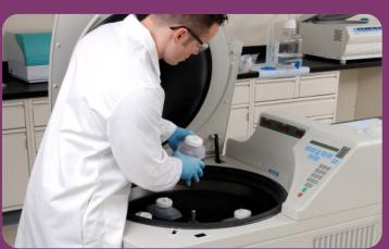
With the H-12000 rotor, you can process up to 12 blood bags with 550mL collection volume each. The high-capacity H-12000 rotor features a corrosion resistant stainless steel body that separates from an aluminum windshield for safe handling and easy cleaning.
