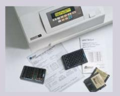
The SpectraTest validation test plates for absorbance and fluorescence intensity provide a complete traceable solution for validating optical performance of the SpectraMax M2 system, automatically.
