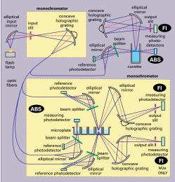
The SpectraMax M2 optical system design provides performance similar to a dedicated spectrofluorometer or spectrophotometer and is the only optical system that has integrated a dual-mode cuvette port and microplate reading
