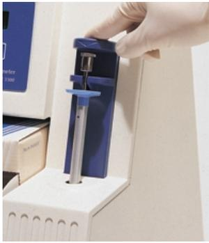
*Operating the Advanced Micro-Osmometer Model 3300 is fast and easy. Once the sample has been aspirated into the sample tube, simply insert the tube into the instrument's vertical holder. Push the holder down and testing begins automatically. Results are displayed in 60 seconds.*
