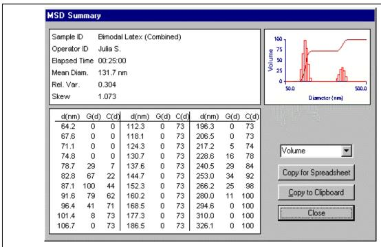
**Figure 2** Bimodal particle size distribution obtained from the **90Plus**. Note that measured values agree with those expected from the prepared suspension.
