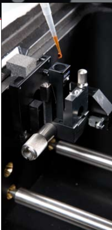
Autosampler for particularly high sample throughput
