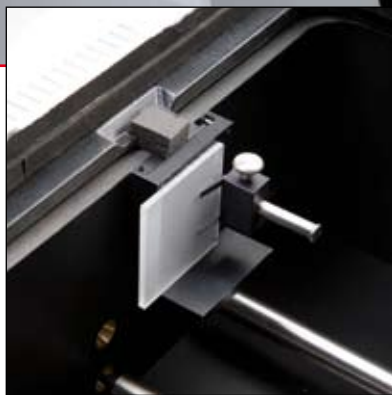
Solid sample holder to determine transmission characteristics
