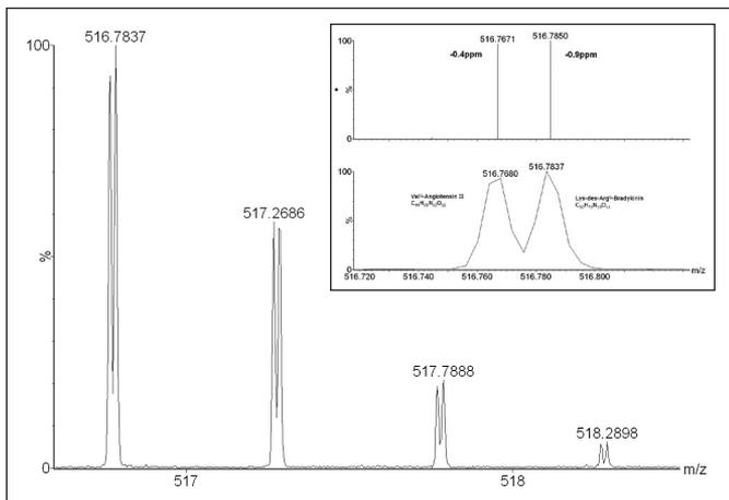
Figure 2. A high resolution oa-ToF spectrum of the isobaric peptides Val5-Angiotensin II and Lys-des-Arg9-Bradykinin.
