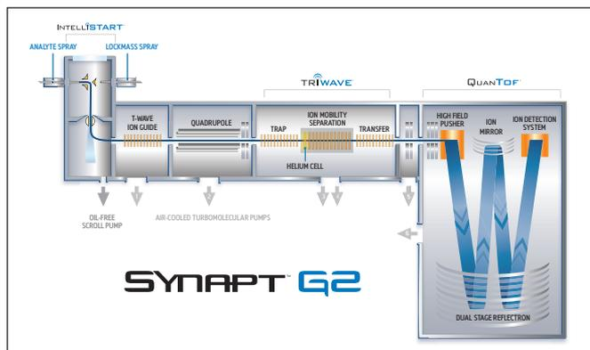
Figure 1. QuanTof Technology, the enabling high-resolution ToF technology of the SYNAPT G2 System:
