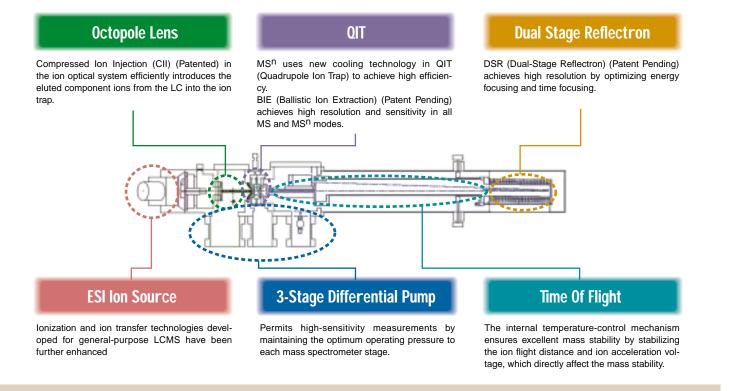
Support for MS<sup>10</sup>; Compressed Ion Injection (Patented) efficiently introduces ions MSn into the ion trap and enhances sensitivity.
