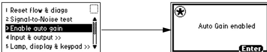
The diagnostic will run during the next injection. The sticky diagnostic (wrench) icon appears on the front panel, and <Auto Gain> appears in the emission field.
