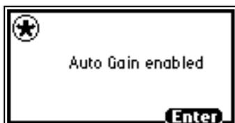
**Tip:** To disable the Auto Gain diagnostic test, press Enter.
