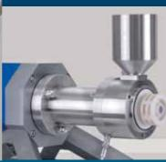
Emptying the grinding beads and cleaning of the grinding chamber is easy to do when the grinding container is dismantled
