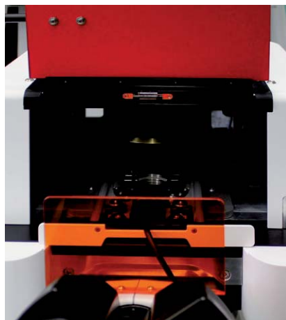
Open NanoTracker™ 2 head with mounted PetriDishHeater™ ▶
