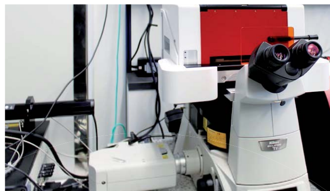
NanoTracker™ 2 mounted on a Nikon Eclipse Ti confocal microscope
