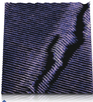
Hexacontane C 60 H 122 on HOPG. Adhesion image (range: 2 nN) measured with QI™ Mode in 3D. Stripes are monomolecular layers of Hexacontane. Scan size: 250 nm × 250 nm, XY closed-loop
