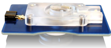
◀ Cantilever holder with electrical tip connection (enclosed volume)
