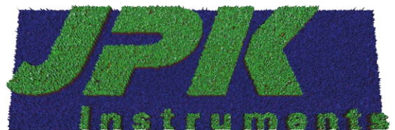
▲ Piezoresponse Force Microscopy (PFM) of ferroelectric polymer (P(VDF-TrFE)) on gold backelectrode on silicon. A sequence of voltage pulses was generated from the grayscale of the JPK-logo bimap template (black = -20V, white = +20V) to write the logo into the samples piezoelectric polarization. 3D vertical PFM-phase (range: 180°), scan size: 12 µm × 30 µm
