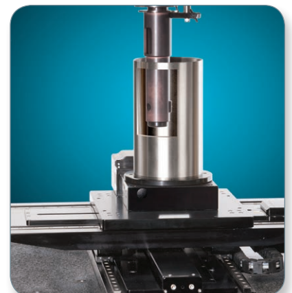
Bore-Scope objective collecting data 150 mm inside large metal engine cylinder liner.
