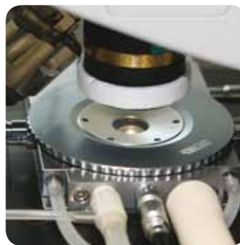
HYPERION sampling stage with internal heating and cooling devices.
