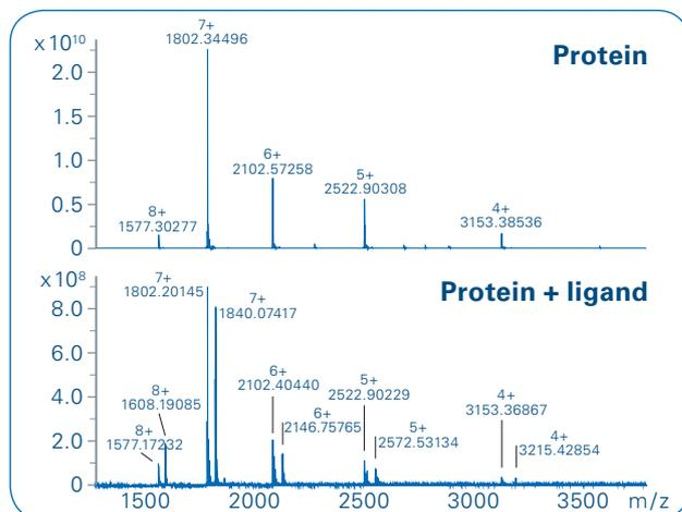
Weak binding ( $K_d > 10 \mu\text{M}$ ) interactions typical in FBDD are routinely preserved and observed by MRMS. The balanced ion optics require no special modifications for native MS.
