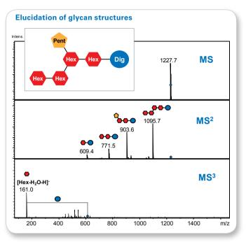
MS<sup>n</sup> enables characterization of digitonin, a steroid glycoside. The complete glycan structure, down to the initial sugar unit, can be elucidated in consecutive MS<sup>n</sup> steps.
