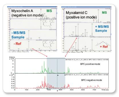
Quick and reliable identification of natural compounds from myxobacteria by library search. Sensitive and highly reproducible MS/MS data allow direct comparison of experimental data with library reference spectra. Fast polarity switching delivers detection of compounds in both ionization modes and ensures that compounds are not missed.
