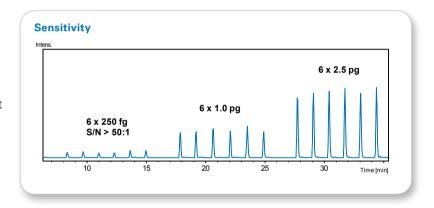
MS/MS sensitivity for multiple injections of reserpine. S/N ratios > 50:1 are reproducibly obtained using 250 fg column loads.
