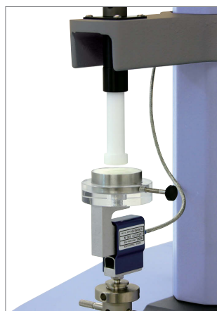
Load cell attached to lower jig
