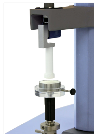
Load cell attached to crosshead
