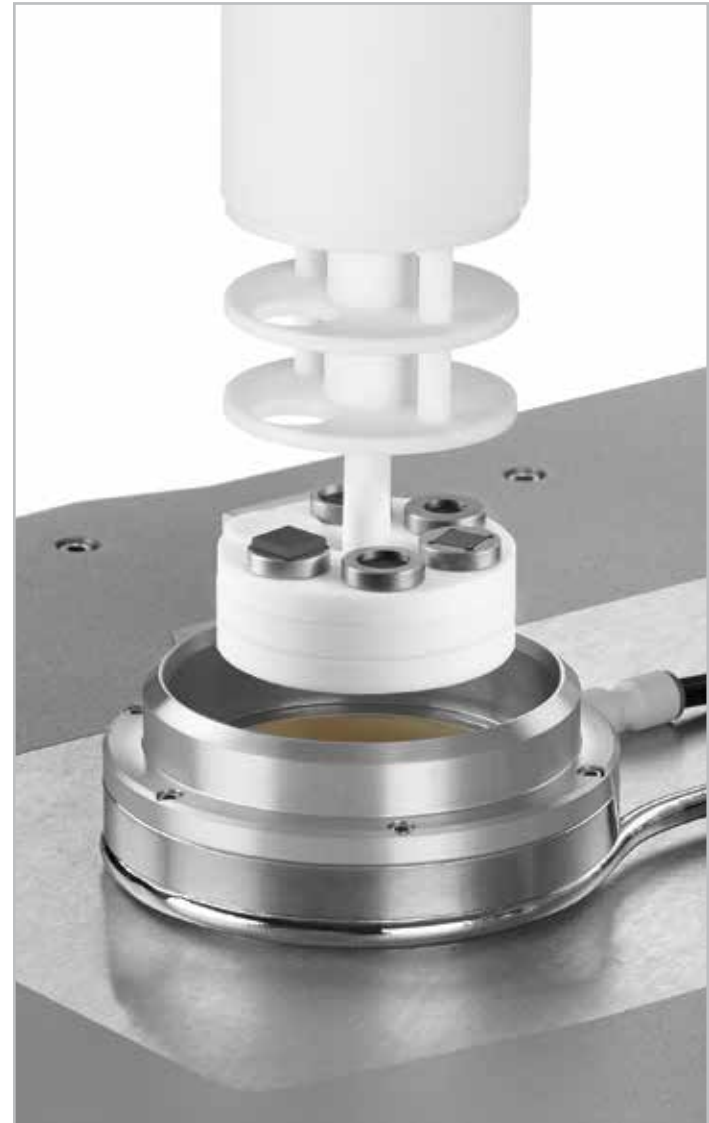
Patented Multi-sample Carousel with Flexible Tray and Adaptors
